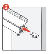
**C.1**Slide trigger into top of track
