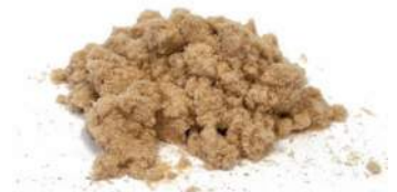
MDF FIBER WITH RESIN
