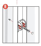
**B.1**Mount panel guide accordingly using the included blockers that fit your glass thickness
